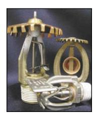
**Suppression-mode sprinklers**, such as Early Suppression, Fast-Response (ESFR) sprinklers are designed to knock down a fire as fast as possible using an aggressive large-drop spray and a flame-penetrating central core of water.
